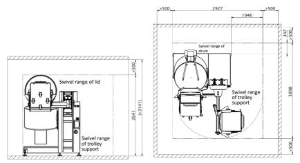
The work area around the machine is at least 0.5 m on all sides; for maintenance work it is at least 1 m; if used as passage way, it is at least 1.2 m.
